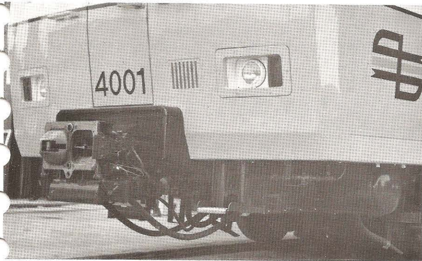
Scharfenberg automatic centre coupler fitted to each end of the twin-body cars. The electric connections include the controls for releasing the plug-type passenger access doors and their closure. The other connections include the hose pipe connection for the main reservoir of the airbrake.
